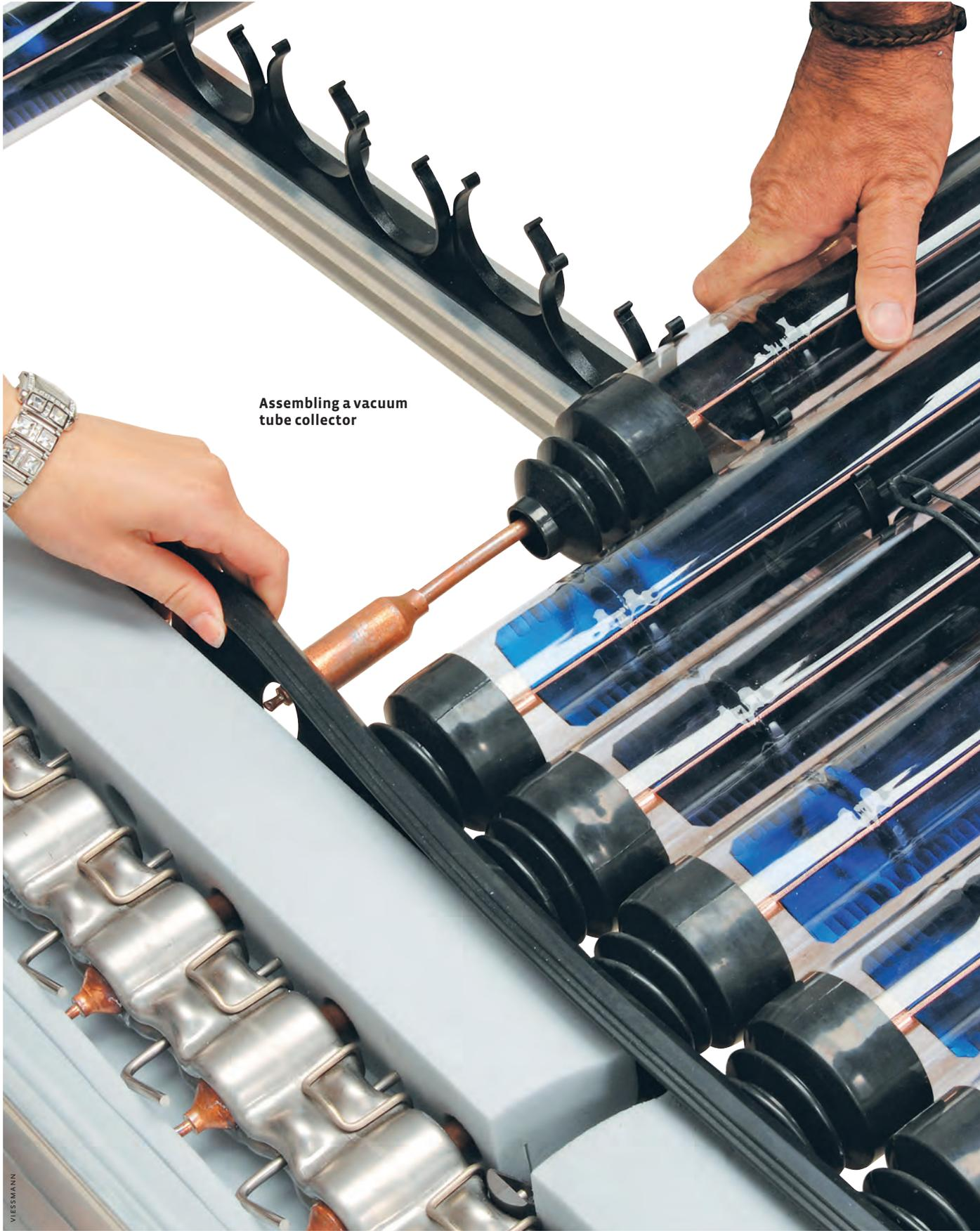
Assembling a vacuum tube collector
