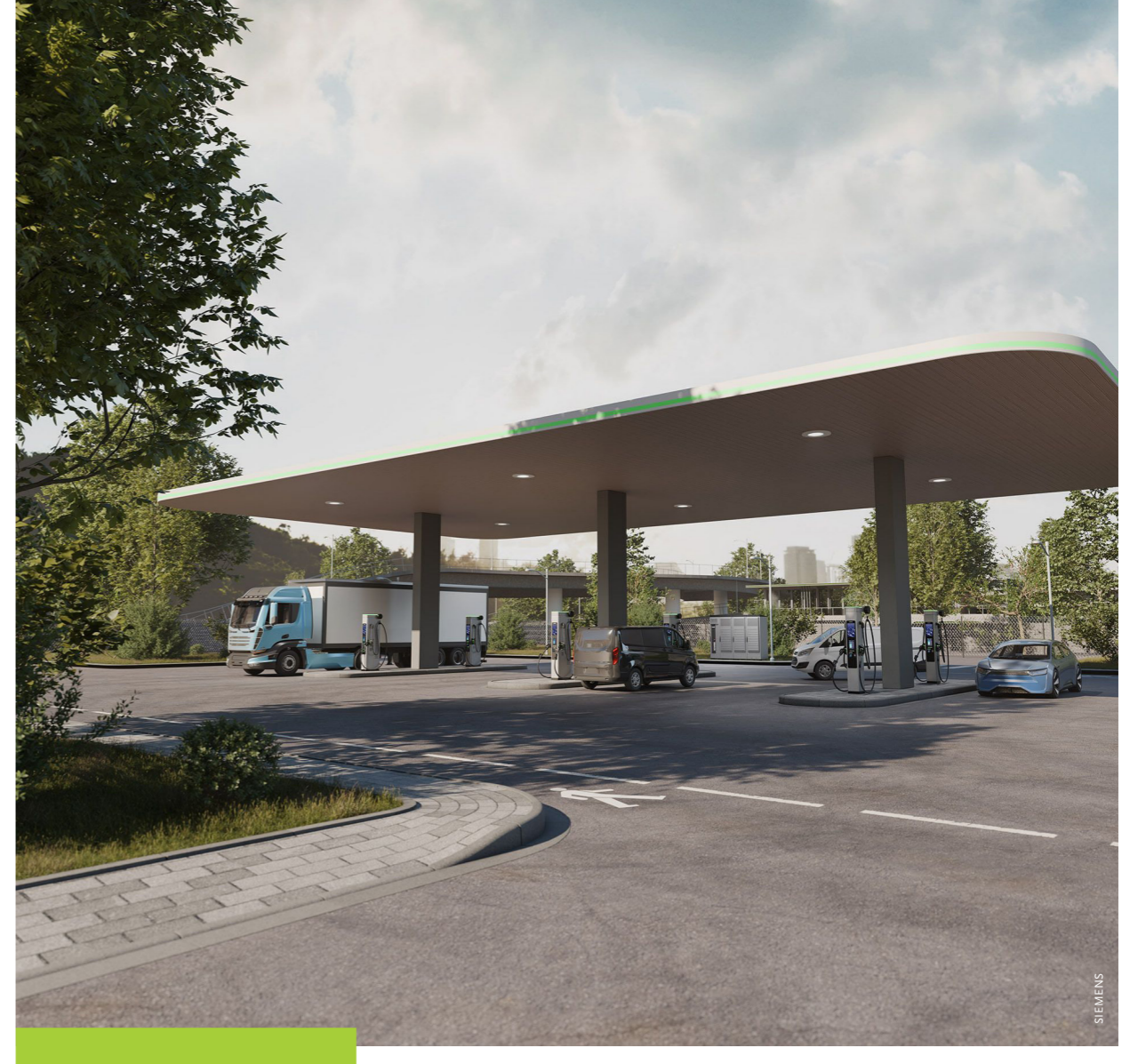
Siemens' Sicharge Flex charging system for electric vehicles can deliver between 480 kW and 1.68 MW. It is compatible with many types of heavy electric vehicles, including trucks and buses.
