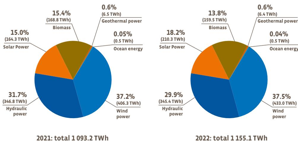
Notes for calculation: Hydro is normalised and excluding pumping. Wind is normalised. Solar includes solar photovoltaics and concentrated solar power generation. Biomass includes electricity generation from solid biofuels, liquid biofuels and biogas (pure and blended in the natural gas grid) calculated according to their compliance with the criteria of Directive (EU) 2018/2001 and also renewable municipal waste. Source: EurObserv'ER from Eurostat database (updated 28 January 2024) and SHARES
