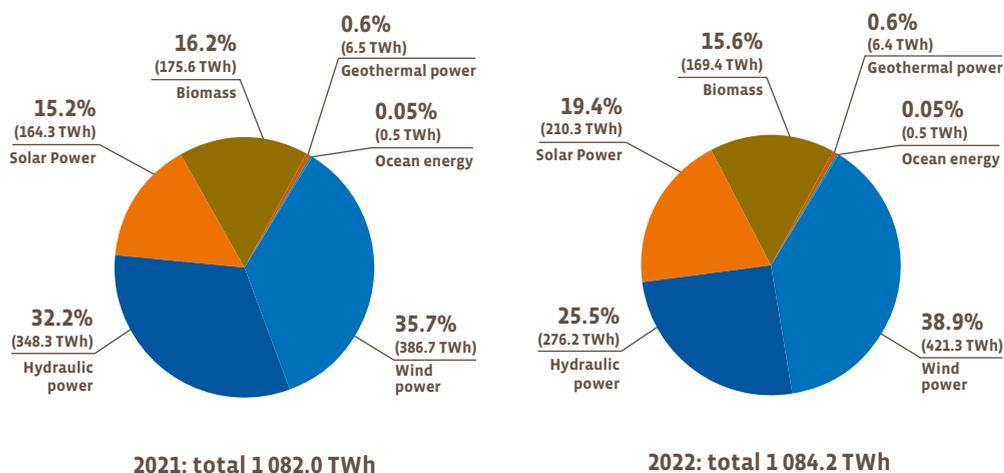
Notes for calculation: Hydro is actual (not normalised) and excluding pumping. Wind is actual (not normalised). All electricity production, compliant or not with renewable Directives, from solid biofuels, biogas (pure and blended in the gas natural grid) and bioliquids is included. Source: EurObserv'ER from Eurostat database (updated 28 January 2024)
