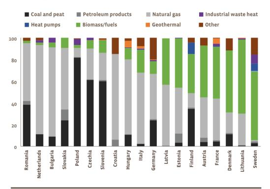
Source: EurObserv'ER - own assessment based on diverse sources. Notes: Based on 2019 data for: BG, DE, EE, FI, SE; 2018 data for: AT, 2017 data for: SK, CZ, SI, HR, HU, IT, LV, FR, DK, LT, PL and data for 2013: RO and NL. Other includes renewable and non-renewable forms of energy such as (non-renewable waste, solar thermal, etc.).
